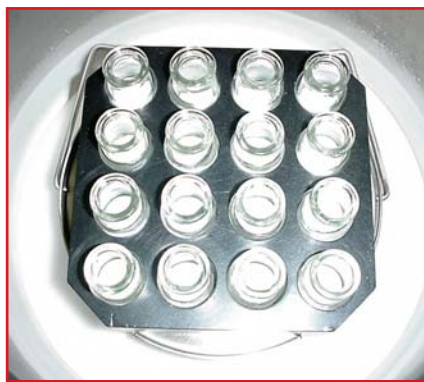
Handle is rotated to raise the shelf to the drying position
