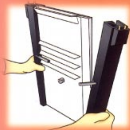
1. Assemble the gel sandwich and slide the lever clamps over the sandwich
