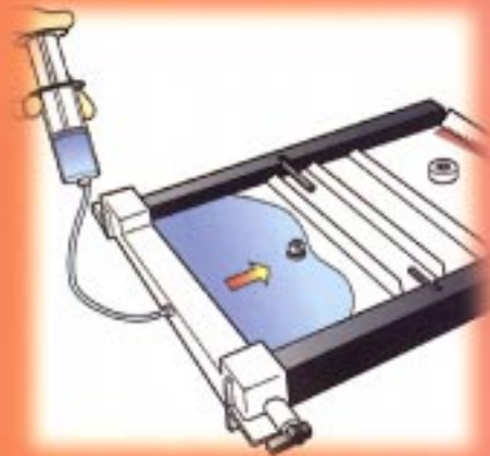
3. Lay the assembly flat, attach the syringe, inject gel solution between the glass plates
